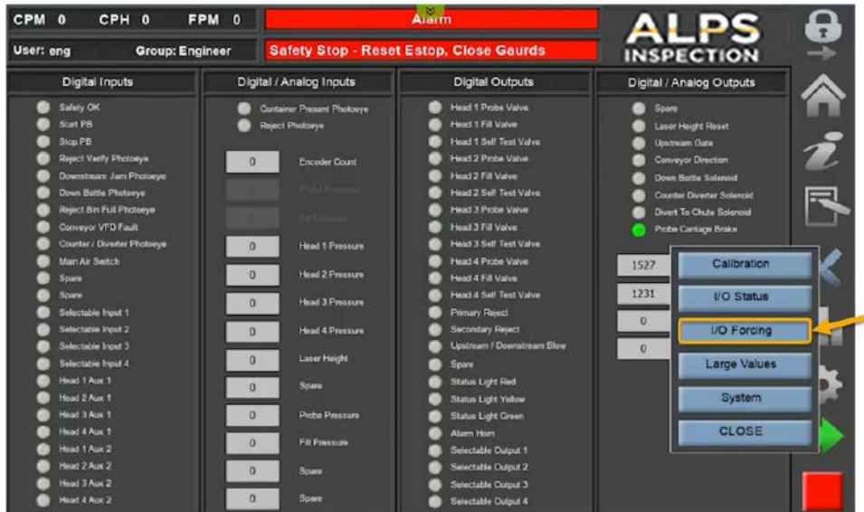
Figure 57: Navigation to I/O Forcing Screen
