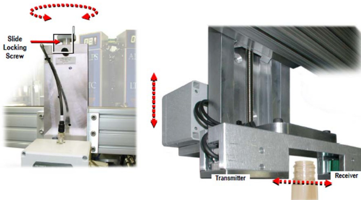
Figure 83: Raise and lower the laser sensor over the container
