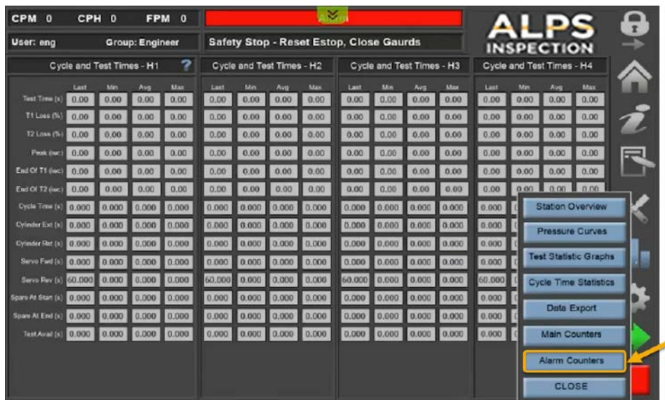
Figure 47: Alarm Counters Menu Navigation
