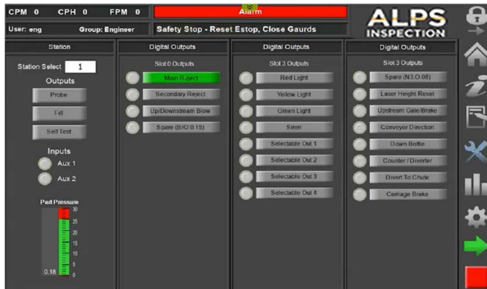
Figure 65: I/O Forcing Screen
