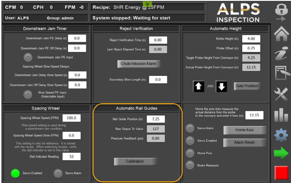
Figure 26: Automatic Rail Guides Screen
