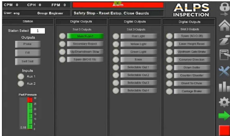
Figure 58: I/O Forcing Screen
