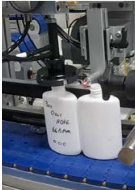
Figure 18: Bottle Line Up with Photo Eye and Probe Example
